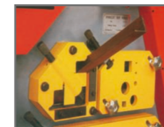
Single shear with no material wastage and minimal deformation. 45° miter-cut is easy and tidy. Static blades have four usable cutting edges. Selectable corner radii on moving blades for optimum results on small or large angle steels.
