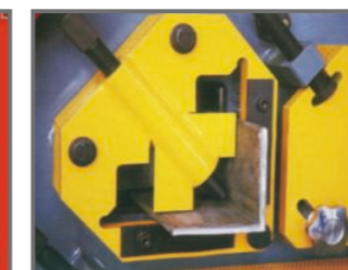
Single shear with no material wastage and minimal deformation. 45° miter-cut is easy and tidy. Static blades have four usable cutting edges. Selectable corner radii on moving blades for optimum results on small or large angle steels.
