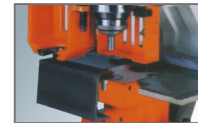
Overhang die holder for punching channel flanges and angles.
